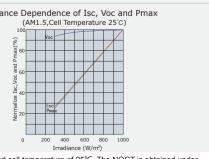
**Note:** the specifications are obtained under the Standard Test Conditons (STCs): 1000 W/m² solar irradiance, 1.5 Air Mass, and cell temperature of 25°C. The NOCT is obtained under the Test Conditions: 800 W/m², 20°C ambient temperature, 1m/s wind speed, AM 1.5 spectrum.
