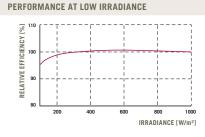
The typical change in module efficiency at an irradiance of 200 W/m<sup>2</sup> in relation to 1000 W/m<sup>2</sup> (both at 25 °C and AM 1.5G spectrum) is -2.5% (relative).
